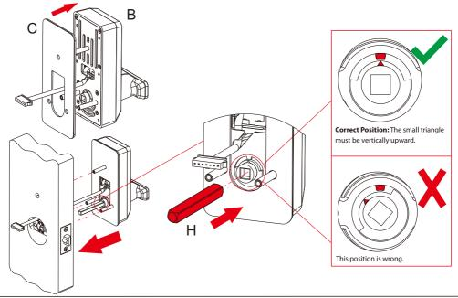
4. Install mounting plate (I) with gasket (C) on the door.
