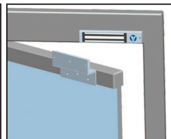
Demonstration of ZL Bracket Installation
