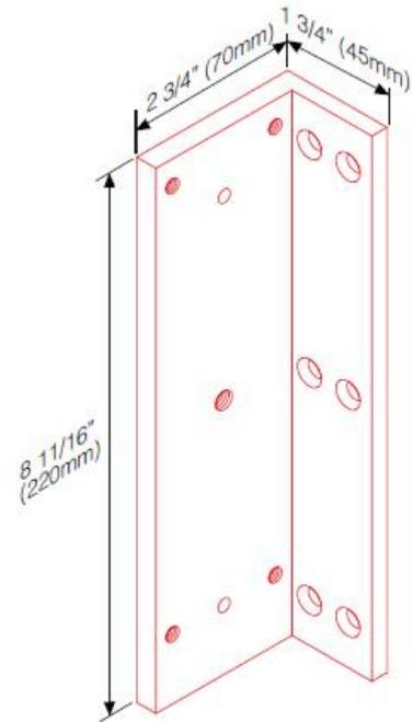
Application for the Electromagnetic: GL-1200F series
