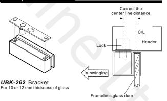
The UBK Bracket can be use on a frameless glass door. With optional 10mm or 12mm depending on the glass thickness. It is suitable for models EB-220 and EB-262. Installations: Fix the strike plate on the UBK-262 Bracket, add silicone for a firm grip on the glass door.
